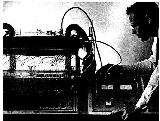
ELECTROPHORESIS, the movement of particles in solution by means of an electric current, is used by molecular biologists at Du Pont to purify proteins in a fundamental research project.
