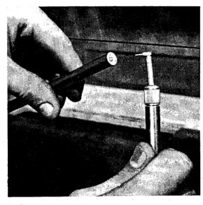
Cleaning the cut-off end of thermocouple assemblies used to be a picky, finicky chore, which took several minutes. It is now done with a two-second pffffft.
