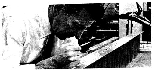
SINE WAVE beams can be accurately welded using a technique developed by Martin Marietta Corp. These beams will be used in the first U.S. supersonic transport.
