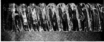
HELICAL 'THREAD' shaped by electron beam in 0.5-in. silica
