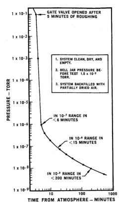
Actual pump down curve for the 18 in. x 30 in. Viton sealed bell jar system shown below. The system was filled with partially dried room air, roughed down, and the gate valve opened at 1 x  $10^{-1}$ Torr. A standard 1600 liter/second Electro Ion pump then produced the results shown above.
