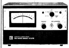
With the new Leeds & Northrup 9838 Guarded Nanovolt Null Detector, you can utilize the full potential of your highest precision potentiometers and bridges. Each 2-mm scale-division of this new solid-state detector can resolve 5 nanovolts at low source resistances and less than 30 nanovolts at 1,000 ohms
