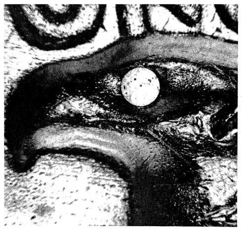
THE TINY black ring in the center of the gold disk is a microminiature varactor produced by Autonetics Div., North American Aviation Inc. It was photographed on the head of an eagle on a U.S. 25¢ piece.
