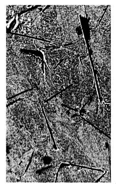
TYPICAL MICROSTRUCTURE graphite within zirconium carbide
