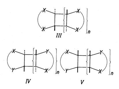
The trans-anti-trans...structure shown in III has several symmetry elements, but it does not contain alternating axes: therefore it exists in two enantiomeric forms. Form III corresponds to the threo-di-isotactic structure of the polymeric chain.
