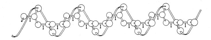
Isotactic polypropylene (contrary to the atactic one, previously known) is a crystalline polymer; it has a high melting point, excellent mechanical properties and can give origin to highly resistant textile fibers and to transparent films.
